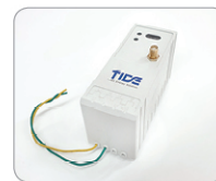
RF Repeater (HPGP PLC 기반)
